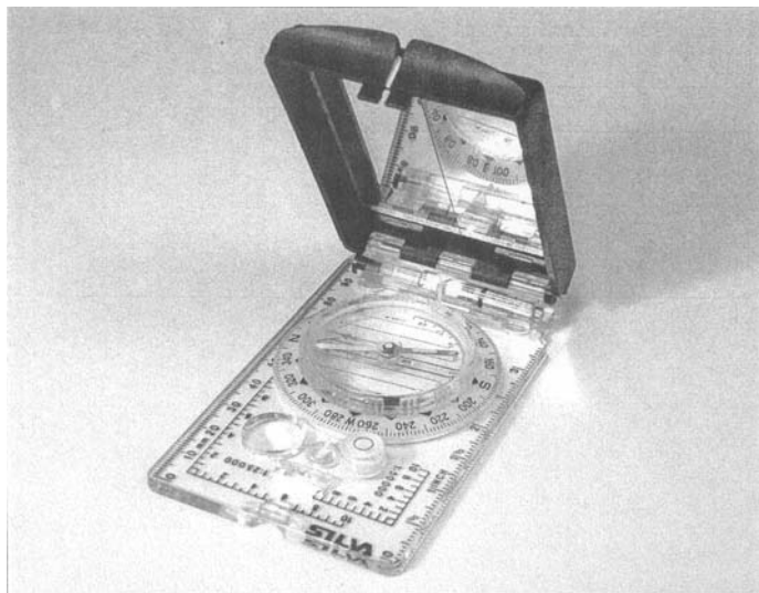
Figure 2.3 The Swedish Silva Ranger 15 TDCL geologist's compass. Like the Suunto, an excellent and reasonably priced instrument
