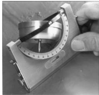
Figure 2.8 Japanese ‘universal clinometer’. Based on the ‘German miner’s hanging compass. Trend can be measured directly from the compass, which always stays horizontal, and plunge is read by the pointer hanging below the compass box
