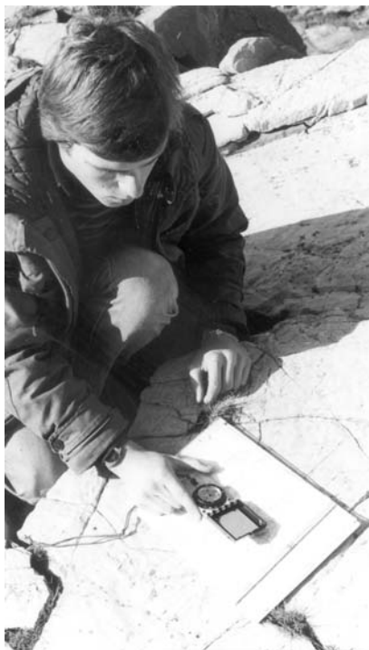
Figure 5.1 Measuring strike by the contact method
